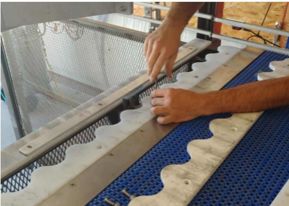
Fig. 34: Fixed Deadplate Removal
