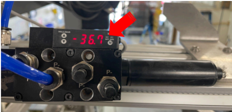
Fig. 10: Vacuum Generator sensor "OUT1" light off
