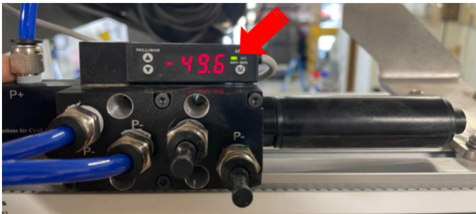
Fig. 11: Vacuum Generator sensor "OUT1" light on
