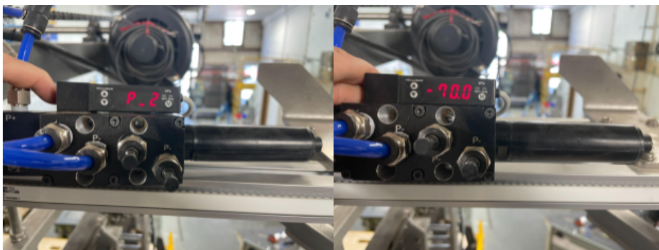
Fig. 9: Vacuum Generator sensor display alternating between "P_2" and current value
