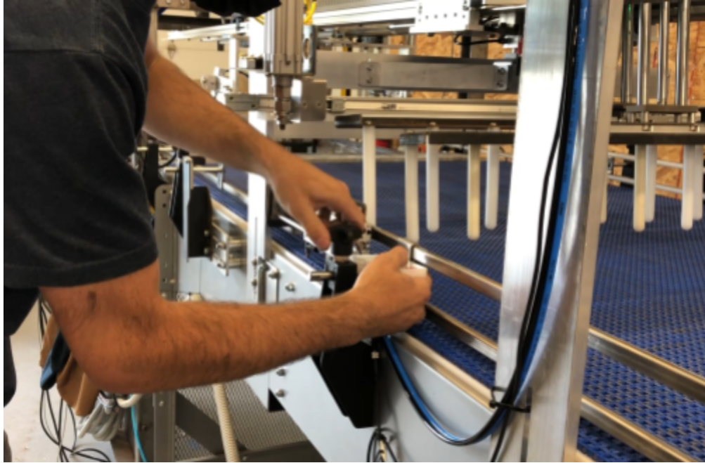
Fig. 39: ValuGuide Rail position adjustment
